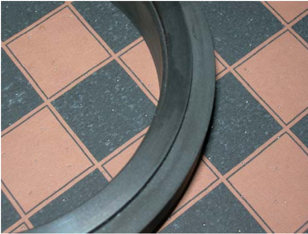
Fig. 7 Inboard stationary seal ring showing very light face wear.
