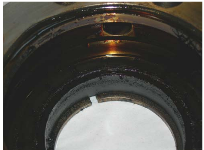
Fig. 4 Outboard stationary seal ring in-situ showing heavy coke deposits and oil tar.
