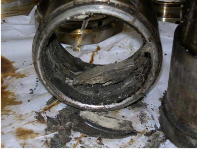
Fig. 5 Spring holder showing heavy scale build up clogging the spring coils.
