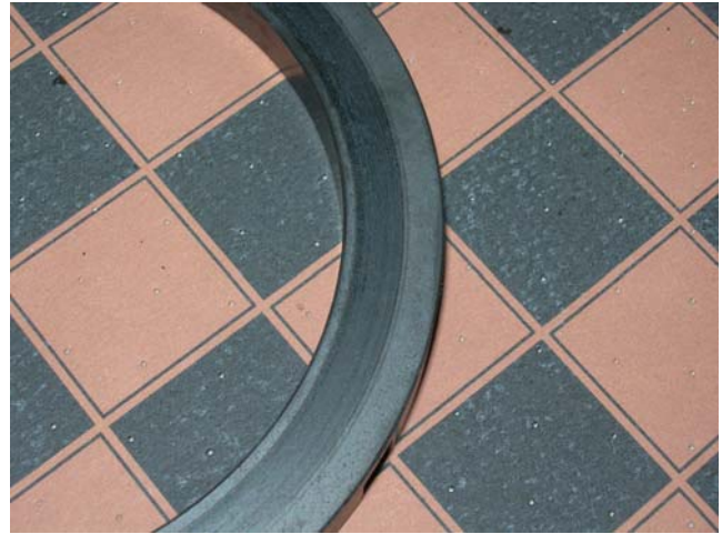
Fig. 8 Inboard rotary seal ring showing very light face wear.
