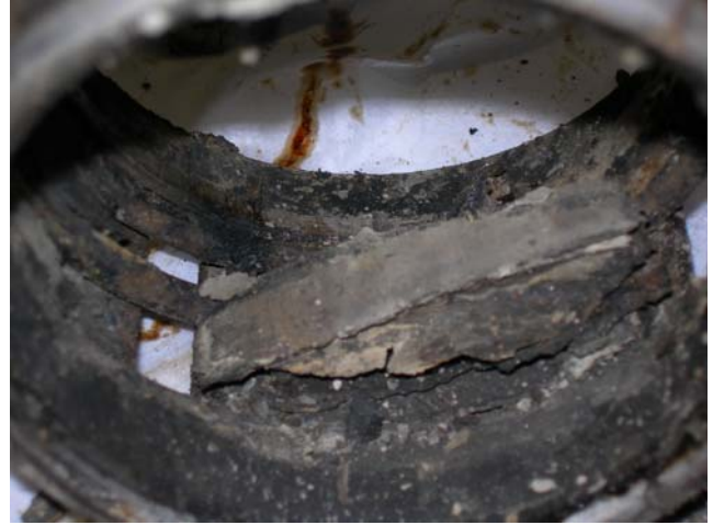
Fig.6 Close up of scale in spring coils.
